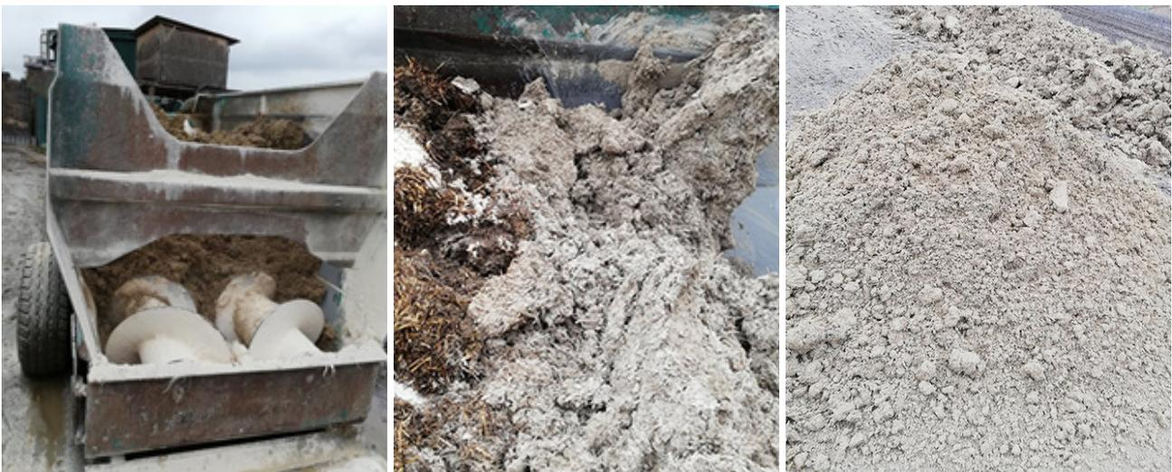
**Figure 2** Production of bedding for dairy cows by mixing components
